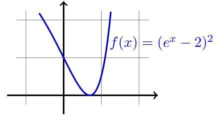
6. Unlike the bisection method, Newton's method will work to find the root of  $f(x) = (e^x - 2)^2$ , but the rate of convergence is not fast. If you start with  $x_0 = 0$ , then even after 10 steps, the approximation  $x_{10}$  is only accurate to two decimal places. Can you explain why Newton's method is so slow? Recall the error formula
